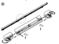
Hook up the leaves to the screws of the tracks, inserting the brackets locations on the screws.
