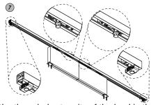
Insert the threaded extremity of the lead in the open loop of the cable fixing bracket and fix it with the corresponding nuts. Fix the cable to the fixing cable brackets with drilled screws, beforehand inserted, and strain it, acting on the nuts assembled on the threaded extremity. N.B. Strain the cable until the two leaves move at the same time.
