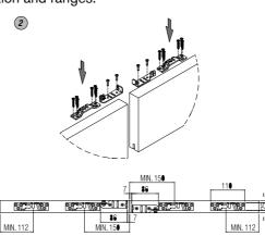
Set the cable around the pulleys and insert the drilled screws on the cable, positioning one screw on the front side and the other one on the back side. Temporarily block the two extremities of the cable on the track with adhesive tape.
