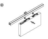
Align the plumb the leaf and fix the inferior adjustable snugs.
