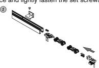
Assemble the fixing brackets leaf and the cable fixing brackets on the panel, respecting the indicated direction and ranges.
