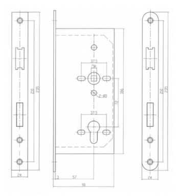
Note: When using a cylinder and turn, if the cam is not fully turned then the lock may jam. We recommend a double cylinder is used with this lock.
