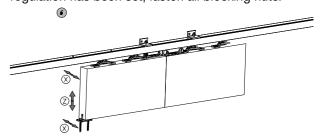
Unscrewing the set screws, on blocking stoppers and adjust the leaves closing. Once the position has been set, definitively fasten the set screws. Set the pulleys at the extremities of the track and definitively fasten the set screws.
